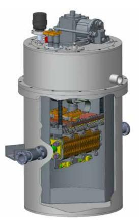
CAD model of the superconducting undulator prototype inside the cryostat.
