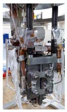
The superconducting undulator prototype before insertion into the cryostat.
